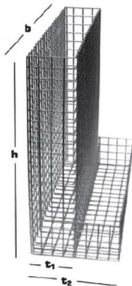
Stahldraht (5 mm), Maschen 50/50 mm
